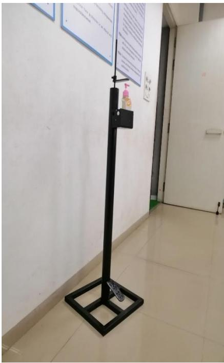
The Department of Mechanical engineering fabricated multiple Hands free Sanitizer Dispenser machine to be deployed in the CMRIT campus as part of the post COVID lockdown measures. The fabrication of the unit was carried out by Mr. Murali and Mr. Krishnappa and is in use on a day to day basis.
